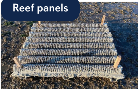
Jute Reinforced Calcium Sulfoaluminate (JR-CSA) in the shape of reef turtles (top), reef prisms (middle), and reef panels (bottom) upon deployment (left) and 6 months (middle) and 18 months (right) post-deployment. Photo courtesy of Mark Clark.
