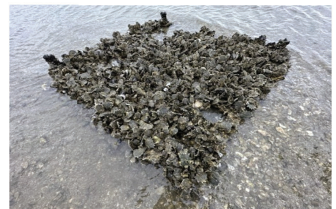
Jute Reinforced Calcium Sulfoaluminate (JR-CSA) in the shape of reef turtles (top), reef prisms (middle), and reef panels (bottom) upon deployment (left) and 6 months (middle) and 18 months (right) post-deployment. Photo courtesy of Mark Clark.
